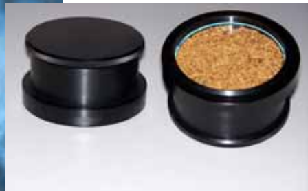
Sample chamber showing underside viewing window & sealed cover
