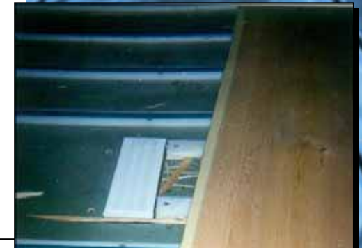
Teflon faced sensor measures hardwood veneer exiting dryer
