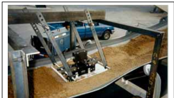
Sled Sensor Measuring Belt Conveyed Aggregate
